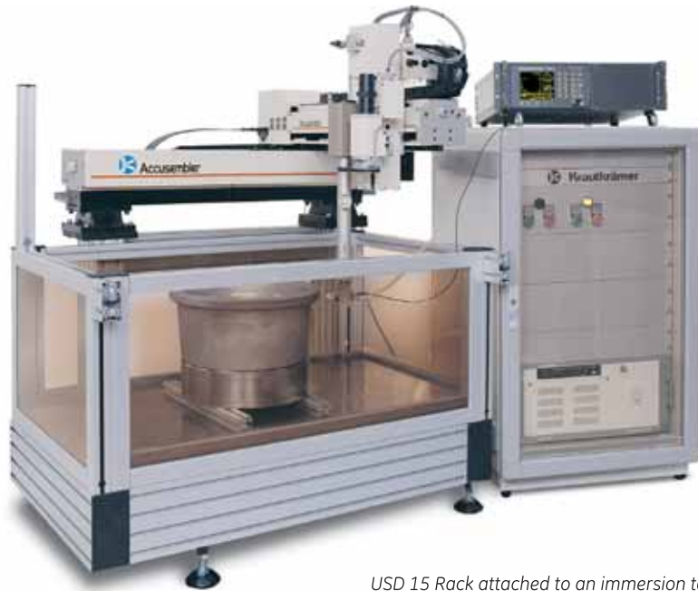
USD 15 Rack attached to an immersion tank
